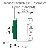
Compact 2 Pushbuttons can be supplied loose or incorporated into stations with 1.5mm or 2.5mm stainless steel faceplates, with a vertical pitch of 50mm and horizontal pitch of 60mm i.e the pushbutton body can be rotated through 90 degrees (horizontal version shown above). If pushbuttons are supplied loose, spacers are provided to accommodate the differing faceplate thickness.
