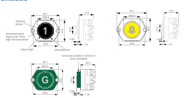
Compact 2 Pushbuttons can be supplied loose or incorporated into stations with 1.5mm or 2.5mm stainless steel faceplates, with a vertical pitch of 50mm and horizontal pitch of 60mm i.e the pushbutton body can be rotated through 90 degrees (horizontal version shown above). If pushbuttons are supplied loose, spacers are provided to accommodate the differing faceplate thickness.
