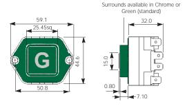
Compact 2 Pushbuttons can be supplied loose or incorporated into stations with 1.5mm or 2.5mm stainless steel faceplates, with a vertical pitch of 50mm and horizontal pitch of 60mm i.e the pushbutton body can be rotated through 90 degrees (horizontal version shown above). If pushbuttons are supplied loose, spacers are provided to accommodate the differing faceplate thickness.
