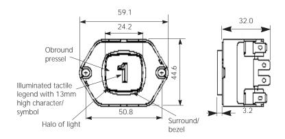
Compact 2 Pushbuttons can be supplied loose or incorporated into stations with 1.5mm or 2.5mm stainless steel faceplates, with a vertical pitch of 50mm and horizontal pitch of 60mm i.e the pushbutton body can be rotated through 90 degrees (horizontal version shown above). If pushbuttons are supplied loose, spacers are provided to accommodate the differing faceplate thickness.
