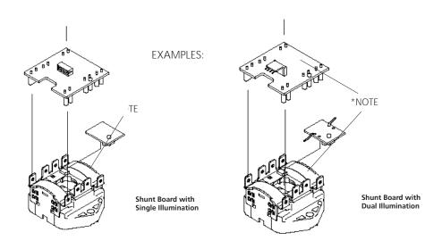
\*NOTE: PCB board must be plugged on to the body with the label (TOP) on PCB on the same side as the Dewhurst logo of the Compact 2 body.
