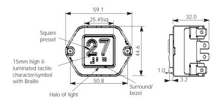
Compact 2 Pushbuttons can be supplied loose or incorporated into stations with 1.5mm or 2.5mm stainless steel faceplates, with a vertical pitch of 50mm and horizontal pitch of 60mm i.e the pushbutton body can be rotated through 90 degrees (horizontal version shown above). If pushbuttons are supplied loose, spacers are provided to accommodate the differing faceplate thickness.
